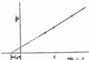
Fig. 11.2. Construction for determination of self-capacitance of coil.
