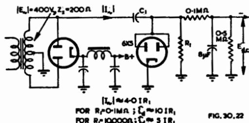
Fig. 30.22. Shunt diode bias supply with r.c. filtering.
