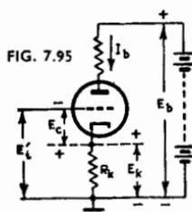
Fig. 7.95. Basic circuit of cathode degenerative triode.
