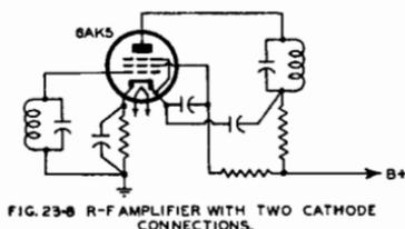
FIG. 23-8 R-F AMPLIFIER WITH TWO CATHODE CONNECTIONS.
