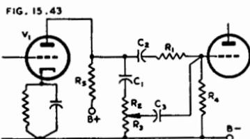
(B) Another example is Fig. 15.43 (Ref. 62) which is capable of giving treble boost 18 db at 10 000 c/s and bass attenuation 6 db at 50 c/s in one extreme position; bass boost 4 db and treble attenuation 21 db in the other extreme.
