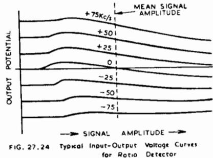
FIG. 27.24 Typical Input-Output Voltage Curves for Ratio Detector
