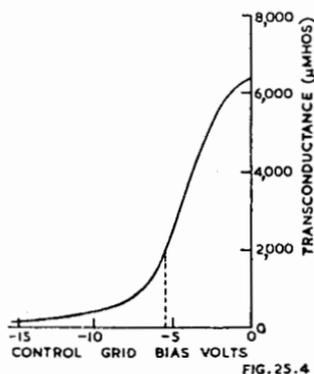
FIG. 25.4. Transconductance characteristic of a typical variable- $\mu$ , radio-frequency pentode.
