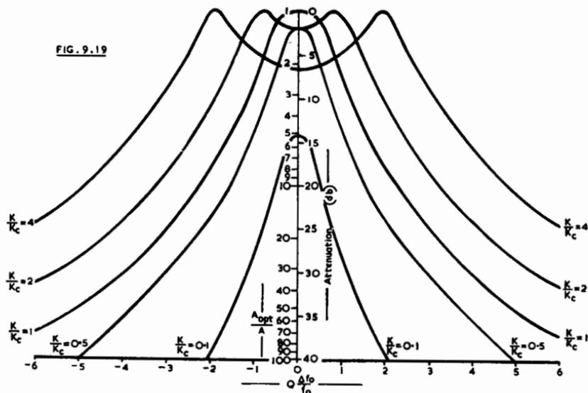
Selectivity Curves for Two Identical Coupled Circuits,
