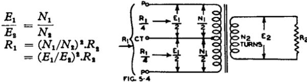
$$\begin{aligned} \frac{E_1}{E_2} &= \frac{N_1}{N_2} \\ R_1 &= (N_1/N_2)^2 \cdot R_2 \\ &= (E_1/E_2)^2 \cdot R_2 \end{aligned}$$
