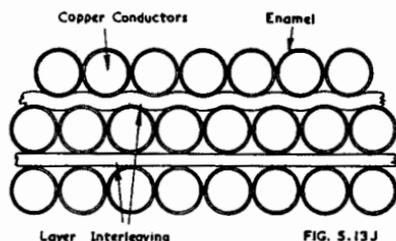
Fig. 5.13J. Section through layer interleaved winding (Ref. C29).
