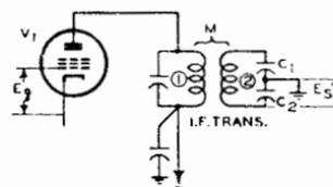
FIG. 26.14 CIRCUIT FOR DETERMINING  $E'_s$
