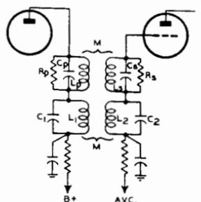
FIG. 26.3 ARRANGEMENT FOR F-M AND A-M I-F STAGE
