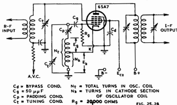
Fig. 25.28. Typical self-excited converter circuit for type 6SA7(GT).
