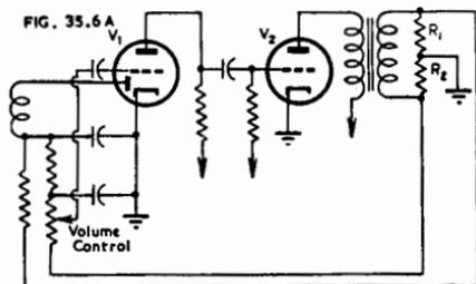
Fig. 35.6A. Combination of positive and negative voltage feedback.
