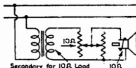
It is important to check for the phasing of the two loudspeakers ; in the vicinity of the cross-over frequency both units should be in phase (aiding one another). This may be checked by the use of a single dry cell connected in series with the secondary of the transformer ; in the case of 2 ohm voice coils there may be a 5 ohm limiting resistor connected in series with the cell.
