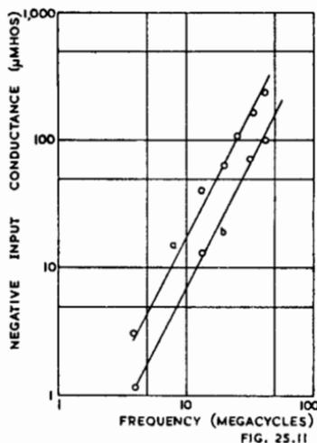
Fig. 25.11. Signal-grid (grid No. 4) conductance of a typical mixer designed for inner-grid injection of oscillator. Lines are drawn with slope of 2. Curve a taken with  $E_c = 0$ ,  $E_4 = -3$  volts. Curve b taken with  $E_{c1} = -6$ ,  $E_4 = -6$  volts.
