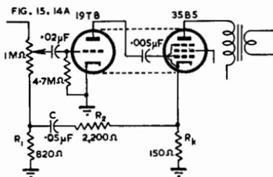
Fig. 15.14A. Two stage amplifier giving 13 db effective bass boost (Ref. 65).
