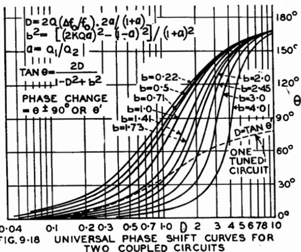
FIG. 9.18 UNIVERSAL PHASE SHIFT CURVES FOR TWO COUPLED CIRCUITS
