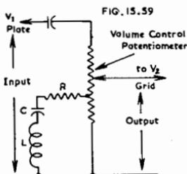
Fig. 15.59. Tone-compensated volume control with tapped potentiometer.
