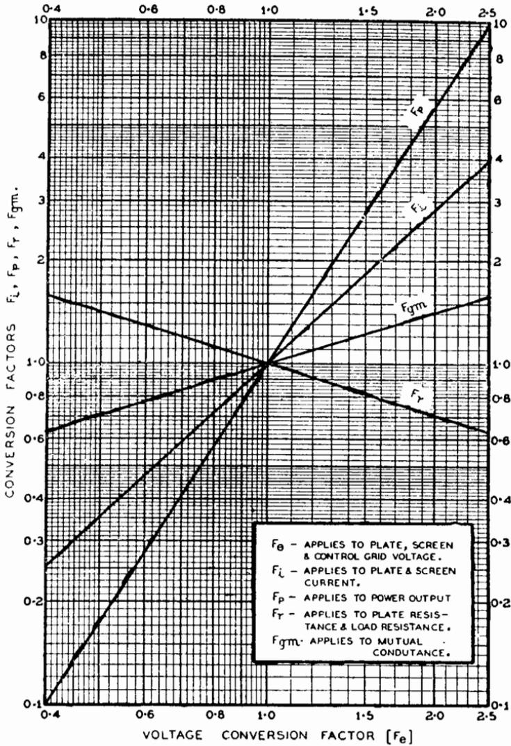
Fig. 2.32A. Conversion factor chart (by courtesy of R.C.A.).
