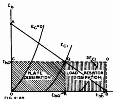
Fig. 2.20. Illustrating power dissipation in a resistance-loaded triode.
