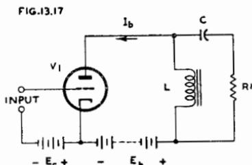
Fig. 13.17. Choke-coupled amplifier.
