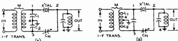
FIG. 26.12 PRACTICAL CIRCUIT ARRANGEMENTS FOR QUARTZ CRYSTAL FILTERS
