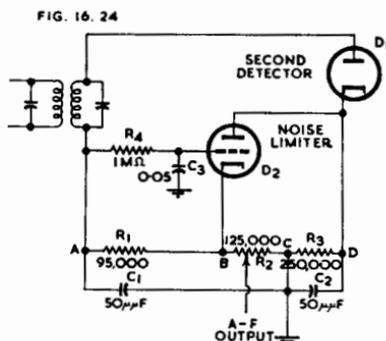
Fig. 16.24. Triode shunt-type noise limiter (Ref. 30).
