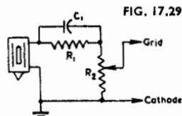
Fig. 17.29. Simple equalizer circuit for a crystal pickup.
