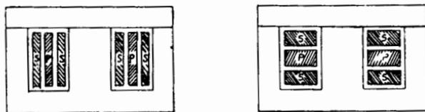
Fig. 5.13A. Typical coil arrangements in audio transformers.
