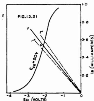
The method is illustrated in Fig. 12.21 where only one plate dynamic characteristic is shown, with a cathode bias loadline OF having a slope of  $-m/(m + 1)R_k$ . The static operating point is at P, the intersection of OF with the dynamic characteristic. Owing to the very large plate load resistors commonly employed, there is very little rise in plate current due to rectification effects, so that P may be regarded as the dynamic operating point.
