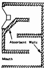
Fig. 20.18. Sectional view of acoustical labyrinth loudspeaker.
