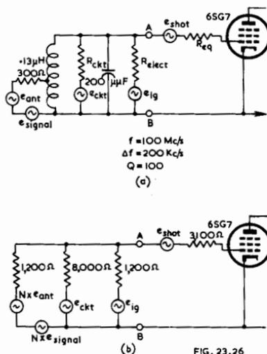
Fig. 23.26. Typical F-M receiver input circuit (Ref. B33).
