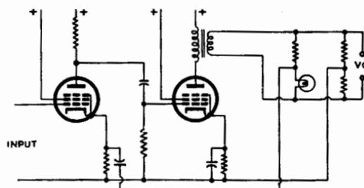
Fig. 16.8. Lamp-operated negative feedback volume expander (Ref. 22).
