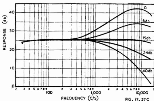
channel. Outputs from the three channels are added in a single valve feedback summing amplifier; potentiometers which add flat loss in the auxiliary channels permit control of the resultant transmission characteristic. The input allows for the connection of two G.E. variable reluctance pick-ups simultaneously. The maximum output is of the order of 1 volt, and the pre-amplifier may be used at a moderately remote location, owing to the cathode follower output.
