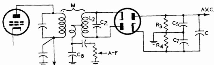
FIG. 27.22 BALANCED TYPE OF RATIO DETECTOR CIRCUIT.
