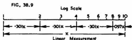
Fig. 38.9. Log. and linear scales (exact).
