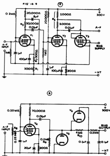
Fig. 16.9. Volume expander using negative feedback; (A) amplifier (B) circuit for supplying control bias to the amplifier (Refs. 22, 24).  $V_1 = V_2 = V_3 = V_4 = 6H6$ ;  $V_5$  and  $V_6$  together = 6H6.
