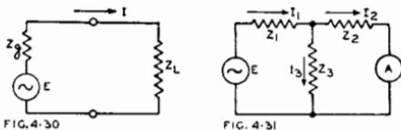
Fig. 4.31. A generator  $E$  supplying voltage to a network, with an ammeter  $A$  to read the current  $I_2$ . The reciprocity theorem states that, when  $A$  and  $E$  are reversed, the transfer impedance  $E/I_2$  will be unchanged.
