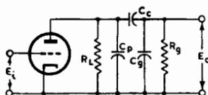
Fig. 7.74. Resistance-capacitance coupled stage.
