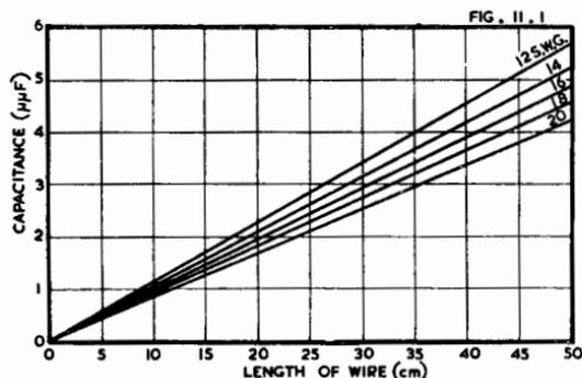
Fig. 11.1. Variation of capacitance with wire length for vertical copper wires of various gauges (Ref. D6).
