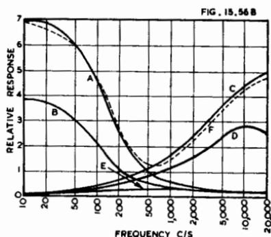
Fig. 15.56B. Response characteristics of Patchett tone control circuit with  $S_1$  closed and  $S_2$  open (Ref. 9).
