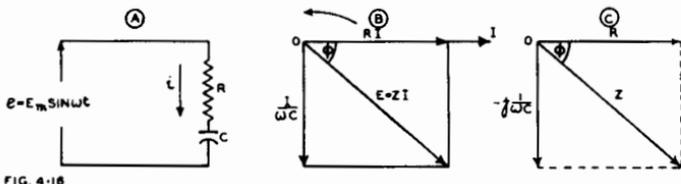
Fig. 4.16. (A) Resistance and capacitance across a.c. line (B) Vector diagram of voltage relationships (C) Vector diagram of impedance ( $Z$ ) with its real component ( $R$ ) and reactive component  $-j(1/\omega C)$ .
