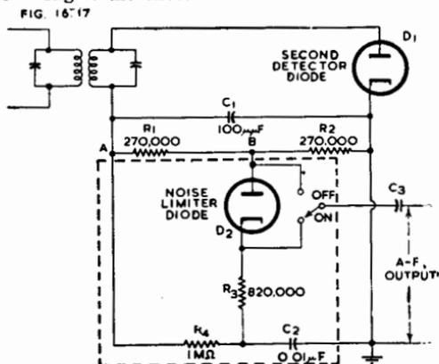
Fig. 16.17. Simple series limiter (Ref. 30).
