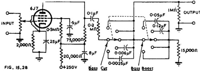
FIG. 15.28. Step-control giving bass boosting and bass attenuation.
