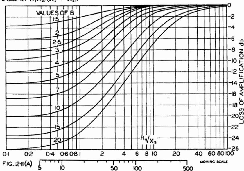
Fig. 12.11A. Curves for the frequency response of a resistance-coupled pentode with screen dropping resistor  $R_s$  and screen by-pass reactance  $X_s$  ( $= 1/\omega C_s$ ). The value of  $B$  is given by eqn. (1a). The frequency for  $R_s/X_s = 1$  is given by  $f = 1/2\pi R_s C_s$ . The frequency scale should be traced and the tracing moved horizontally until  $f$  corresponds to  $R_s/X_s = 1$  (method after Sturley).
