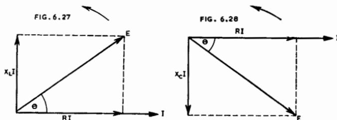
A similar procedure applies with a capacitance instead of an inductance (Fig. 6.28) except that the capacitive reactance is  $X_C$  instead of  $X_L$  and the vector of peak voltage drop across  $C$  ( $X_C I$ ) is drawn vertically downwards, since it must be opposite to  $X_L I$ . The current ( $I$ ) here leads the voltage ( $E$ ) by the angle  $\theta$ .
