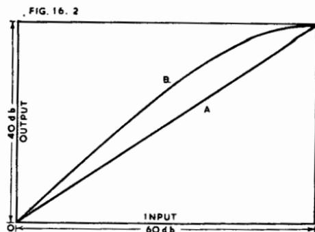
Fig. 16.2. Compression characteristics of volume compressors.
