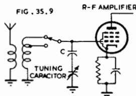
Fig. 35.9. Series-capacitor method of bandspreading.
