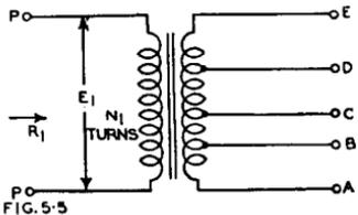
$$\begin{aligned} R_1 &= (N_1/N_{AB})^2 \cdot R_{AB} \\ \text{or } R_2 &= (N_1/N_{BD})^2 \cdot R_{BD} \\ &\text{and so on.} \end{aligned}$$
