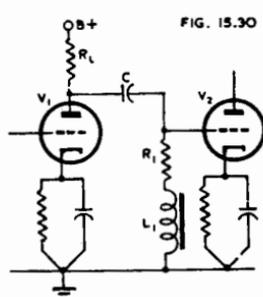
Fig. 15.30. Treble boosting with inductance in grid circuit.
