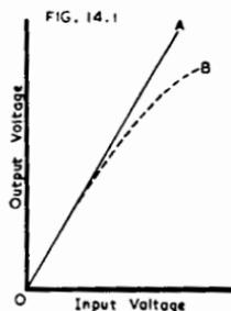
Fig. 14.1. *Linearity characteristic (or transfer characteristic)*
