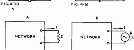
Fig. 4.32. (A) An impedance  $Z$  in a network with current  $I$  and voltage drop  $ZI$  (B) Equivalent circuit having identical results so far as current and voltage drop are concerned, with a generator developing a voltage  $E = ZI$ . This illustrates the Compensation Theorem.
