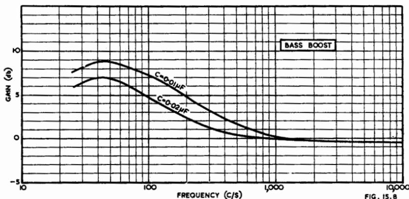
Fig. 15.8. Frequency characteristics with the circuit of Fig. 15.7,  $V_1 = 6J7$ ,  $R_L = 0.05 M\Omega$ ,  $R_1 = 0.2 M\Omega$ ,  $R_k = 2000 \Omega$ ,  $C_k = 25 \mu F$ ,  $R_s = 1.5 M\Omega$ ,  $C_s = 0.1 \mu F$ ,  $C = 0.02 \mu F$ ,  $R_o = 1 M\Omega$ .
