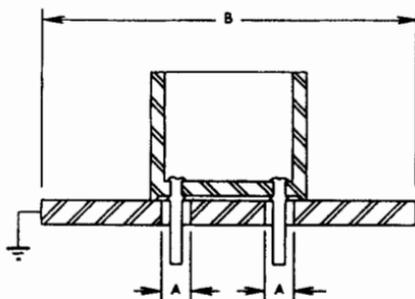
Fig. 3.4A. RMA-NEMA Standard Capacitance Sockets (Ref. S8).
