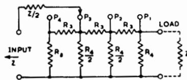
Fig. 18.14. Modified form of ladder attenuator.
