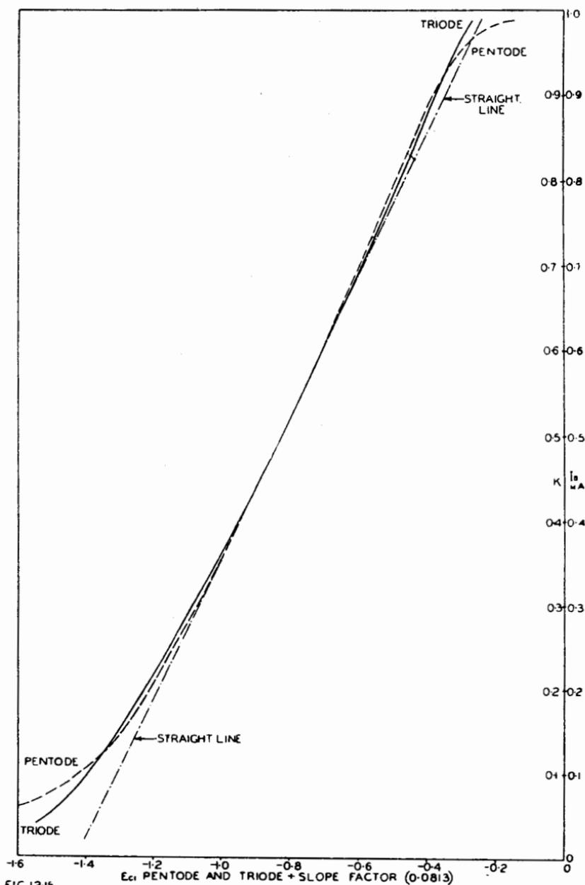
Fig. 12.15. Comparison between pentode and triode dynamic characteristics of the same valve (6SJ7 with  $E_{b,b} = 250$  volts,  $R_L = 0.25$  megohm,  $E_{c2} = 22.5$  volts for pentode,  $E_{c2}$  connected to plate for triode characteristics; triode characteristics divided by slope factor 0.0813 and superimposed so that points for  $I_b = 0.5$  mA coincide).
