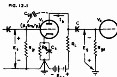
Fig. 12.1. Triode valve ( $V_1$ ) resistance-capacitance coupled to  $V_2$ .
