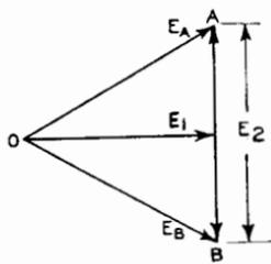
assumed constant for the moment) alters, the phase angle between  $E_1$  and  $E_2$  changes from that at resonance. This leads to a change in the relative magnitudes of  $E_A$  and  $E_B$ .
