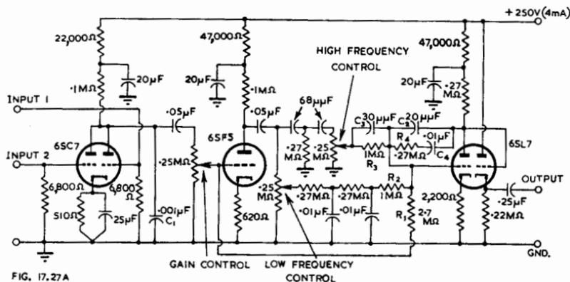
Fig. 17.27. (A) Circuit of continuously variable equalizing pre-amplifier (B) Variation in attenuation in low frequency control (C) Variation in attenuation in high frequency control (Ref. 246).
