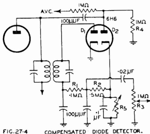
FIG. 27-4 COMPENSATED DIODE DETECTOR.
