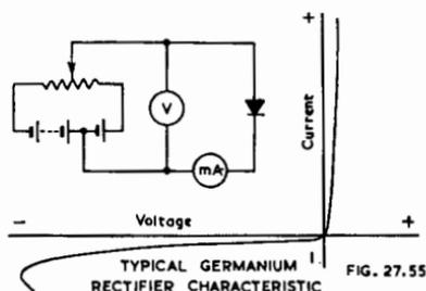
There is little change in rectifier characteristics from 15°C to 50°C, but above this temperature up to 100°C, both forward and back slope resistances decrease slowly.
