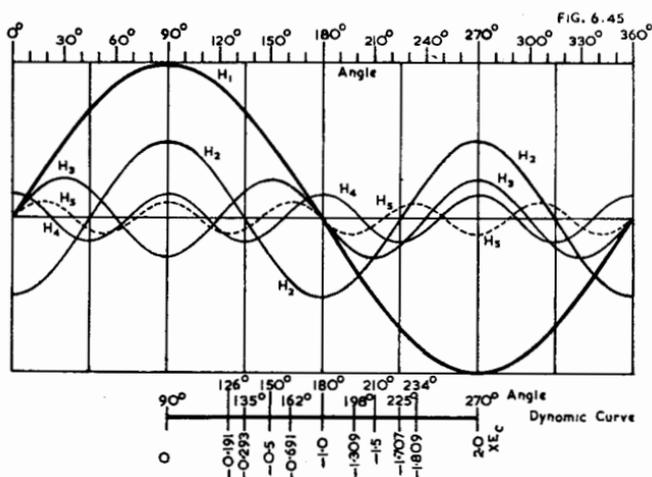
fourth, and higher order even harmonics reach their maximum values (either positive or negative) at  $0^\circ$ ,  $90^\circ$ ,  $180^\circ$ ,  $270^\circ$  and  $360^\circ$  on the fundamental scale.
