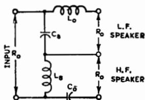
Fig. 21.8. Filter type frequency dividing network, series connection.
