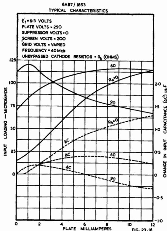
The hot input conductance of a valve with an unbypassed cathode resistor can be determined by modification of the values of  $k_h$  in the table. The value of  $k_h$  in the table should be multiplied by  $g_m/(1 + g_m R_k)$ . The resultant value of  $k_h$ , when substituted in eqn. (1), with  $k_e$  from the table, gives the input conductance of a valve with an unbypassed cathode resistor. In the factor  $(1 + g_m R_k)$ ,  $g_m$  is the grid-cathode transconductance when  $R_k$  is by-passed.
