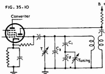
Fig. 35.10. Bandsread circuit to give linear scale.
