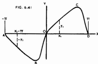
This is the equation for the condition when the fundamental and all the harmonics commence together at zero.
