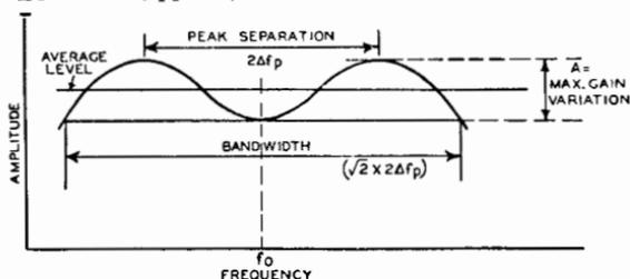
FIG. 26-5 ILLUSTRATION OF TERMS USED FOR OVER-COUPLED TRANSFORMERS
