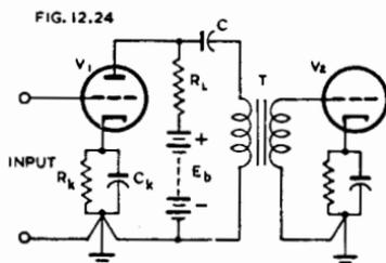
Fig. 12.24. Circuit diagram of parallel-fed transformer-coupled voltage amplifier.
