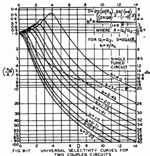
FIG. 9.17 UNIVERSAL SELECTIVITY CURVES FOR TWO COUPLED CIRCUITS
