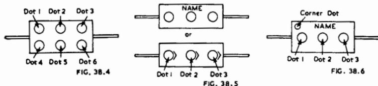
Fig. 38.4. Colour code for moulded mica capacitors (6 dot).
