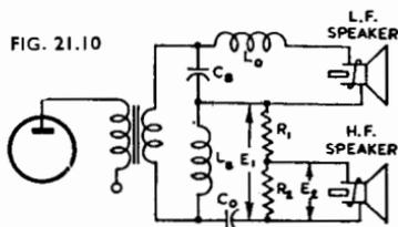
If it is desired to use this as a variable attenuator to give tone control, it should preferably be of the constant input impedance type such as the  $L$  pad [Fig. 21.11, also see Chapter 18 Sect. 3(iii)]. If a simpler type must be used, it may be designed as for Fig. 21.10 to give the correct input impedance at the normal operating position, but with a sliding contact. It will then have an incorrect impedance at any other
