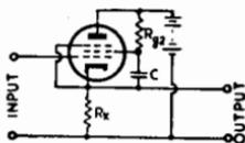
If it is desired to obtain pentode operation, the voltage between screen and cathode must be maintained steady and free from signal frequency fluctuations. This may be done by connecting an impedance (either a voltage dropping resistor or a choke) between the plate and the screen, and by-passing the screen to the cathode by means of a sufficiently large capacitance (Fig. 7.16).
