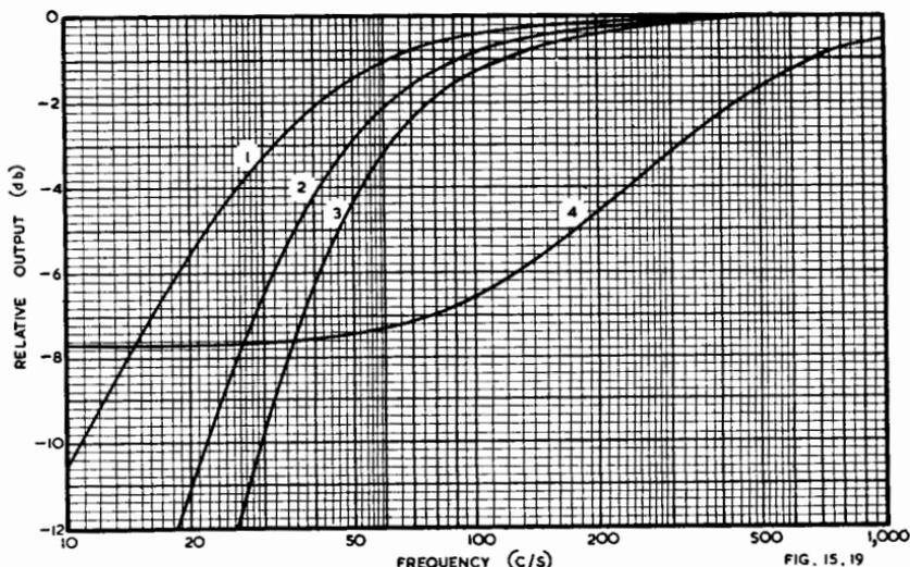
Fig. 15.19. Bass attenuation versus frequency characteristics: (1) Single grid coupling condenser ( $R = 1$  megohm,  $C = 0.005 \mu F$ ); (2) Two stages each with identical values of time constant  $RC$ ; (3) Three stages each with identical values of time constant; (4) R.c.c. pentode with by-passed cathode resistor (6J7,  $R_L = 0.25 M\Omega$ ,  $R_k = 2000 \Omega$ ,  $C_k = 0.5 \mu F$ ) and screen adequately by-passed.
