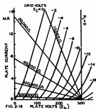
Fig. 2.16. Triode plate characteristics with loadlines for five values of load resistance.
