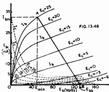
Fig. 13.48. Plate and grid characteristics of a typical small battery-operated Class B triode (1J6-G).
