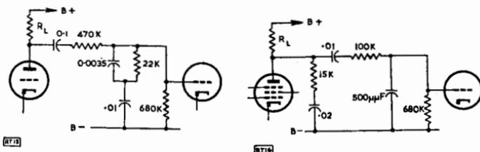
Fig. 17.15E. Equalizing circuit following a triode (RT15).
