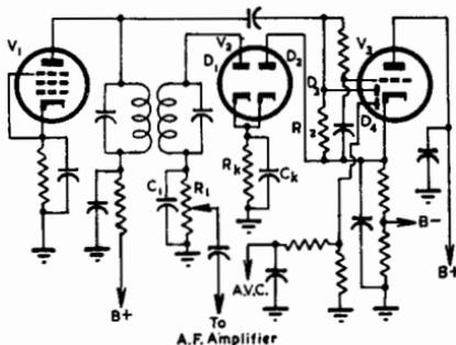
FIG. 27.43 Biased Detector Muting System
