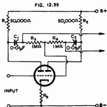
Fig. 12.35. Modified "see-saw" self-balancing phase inverter (Ref. C10).
