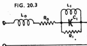
The impedance so far discussed is called the "free" impedance; there is also the "blocked" impedance which is measured with the voice coil prevented from moving. The "motional" impedance is found by a vector subtraction of the "blocked" from the "free" impedance. The difference between the free and blocked impedances is small except in the vicinity of the bass resonant frequency, where the motional impedance becomes the major portion of the free impedance (Refs 13, 41).
