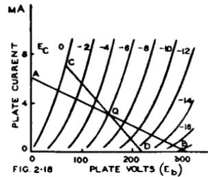
Fig. 2.17. Loadline is independent of valve curves.
