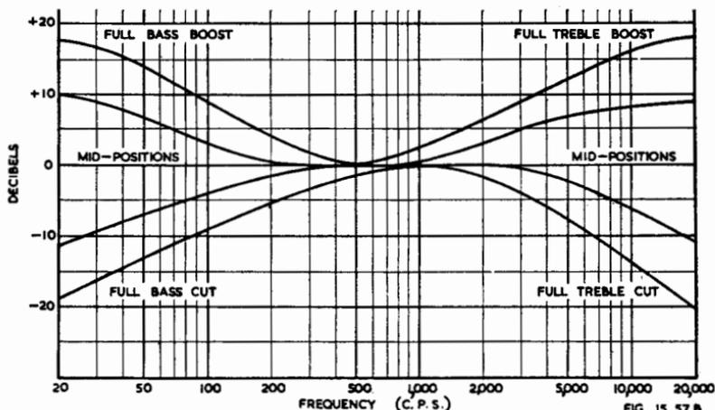
Fig. 15.57B. Response characteristics of Fig. 15.57A (Ref. 77).
