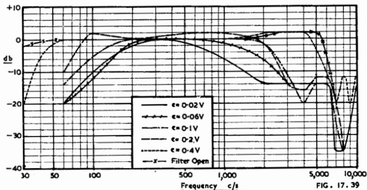
Fig. 17.39. Frequency characteristics of circuit of Fig. 17.37 (Ref. 251).
