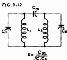
Fig. 9.12. High impedance capacitive coupling.
