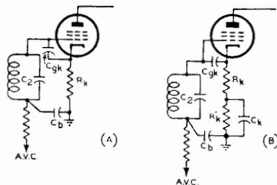
FIG. 26.18 METHOD FOR REDUCING VARIATIONS OF INPUT ADMITTANCE
