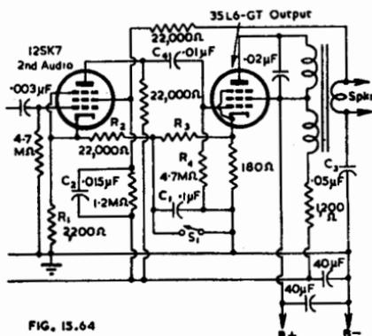
FIG. 15.64. Amplifier providing synthetic bass (Ref. 73).
