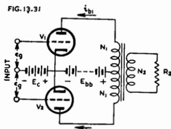
Fig. 13.31. Fundamental circuit of push-pull power amplifier.
