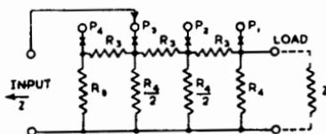
Fig. 18.13. Ladder attenuator ( $\Pi$  section).
