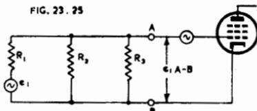
Fig. 23.25. Circuit for reflecting various voltages to the grid (Ref. B33). To find the effective voltage of the antenna, the tuned circuit, and the induced grid noise at the grid of the tube let  $R_1$  equal one of the above noise resistances and  $e_1$  its generated voltage. If  $R_2$  and  $R_3$  equal the other two noise resistances the effective voltage at the grid is
