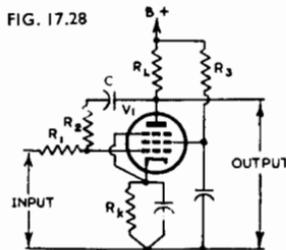
A modification of the circuit of Fig. 17.28 is described in Ref. 280 which gives both bass boosting (with a "very low frequency roll-off") and high frequency de-emphasis. Values of components are:  $R_1 = 0.33$  megohm,  $R_2 = 1.0$  megohm,  $R_L = 0.22$  megohm,  $C = 600\text{ }\mu\text{F}$  approx. (adjustable),  $C_2 = 25\text{ }\mu\text{F}$  approx. (adjustable) shunted across  $R_2$ , and  $V_1 = 6F37$ .
