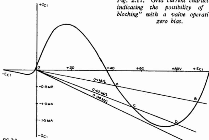
Fig. 2.11. Grid current characteristics indicating the possibility of "grid blocking" with a valve operating at zero bias.
