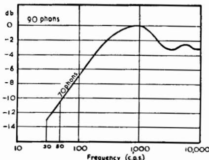
Fig. 14.9. Loss of bass and high audio frequencies caused by reproduction at a loudness of 70 phons as compared with the original at 90 phons (based on Fig. 19.7).
