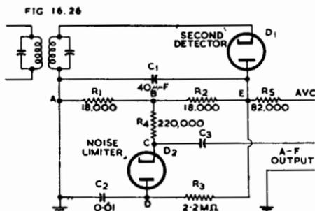
Fig. 16.26. Modified shunt noise limiter (Ref. 30).
