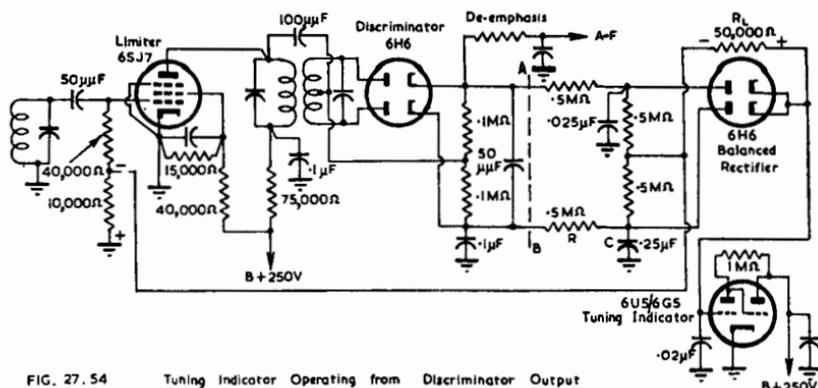
FIG. 27.54 Tuning Indicator Operating from Discriminator Output
