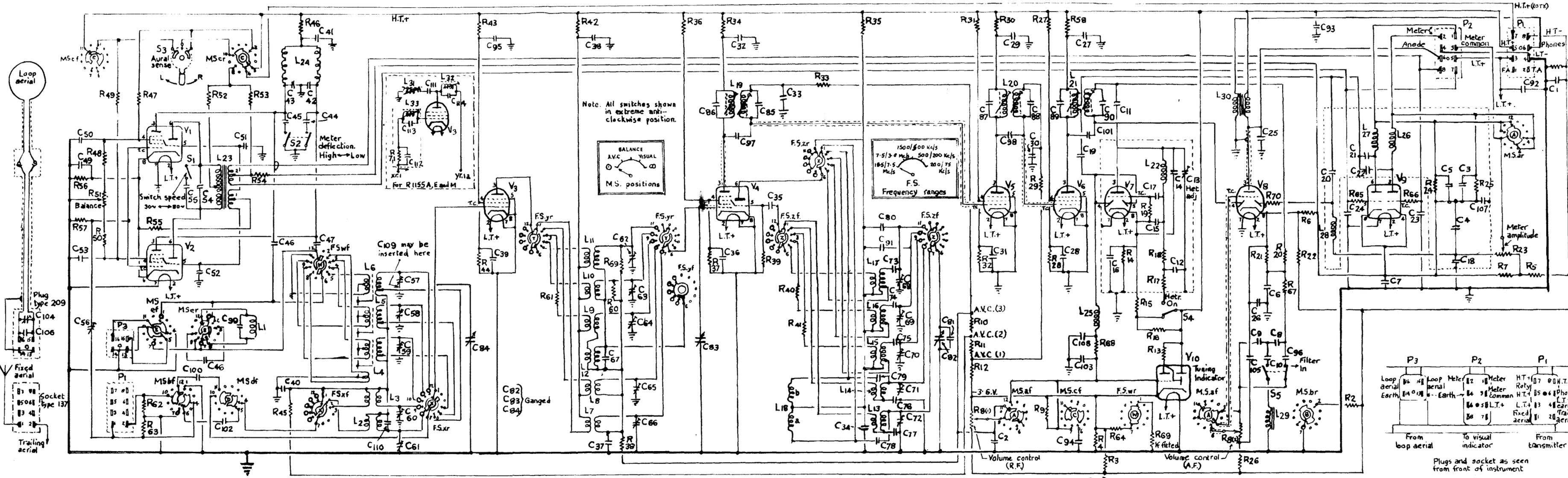
R.1155 AND R.1155D CIRCUIT DIAGRAM INCLUDING R.1155A, R.1155E, AND R.1155M MODIFICATIONS
