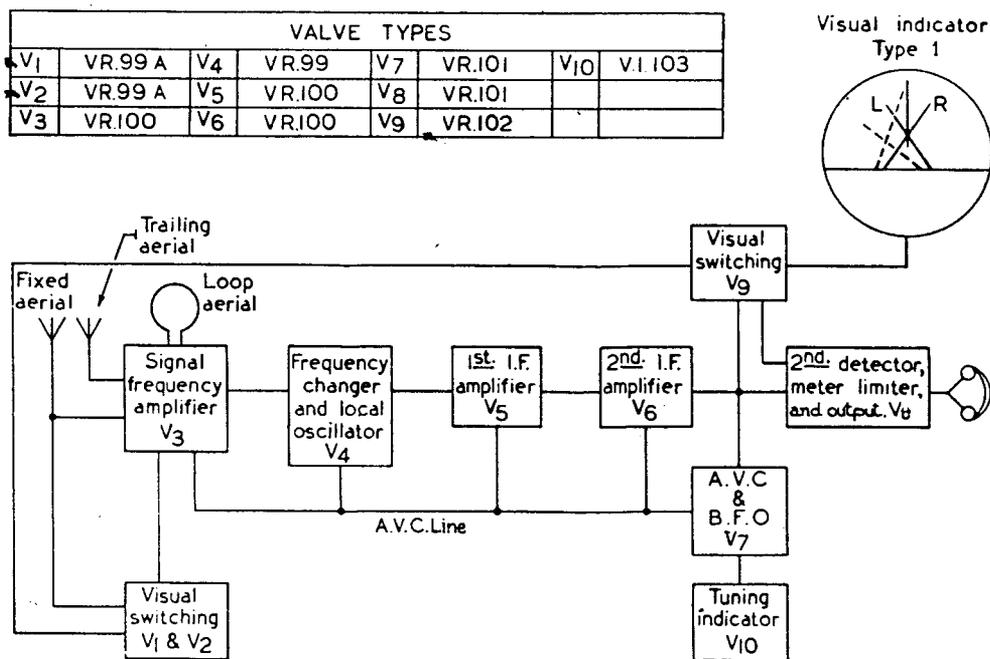
FIG. 2.—SCHEMATIC DIAGRAM
