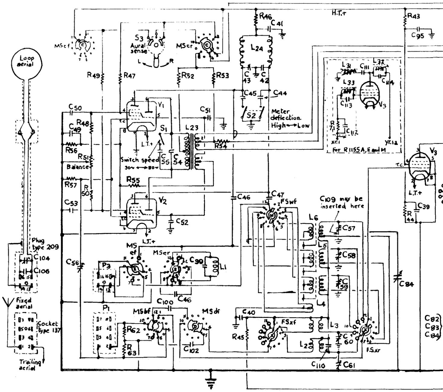
Note. Switch contacts shown thus O, denote front (f) a rear (r) contacts connected. Important. In order to avoid excessive crossing of connecting wires certain switch wafers have been duplicated.
