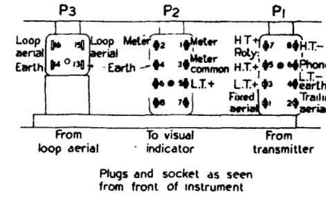
Plugs and socket as seen from front of instrument
