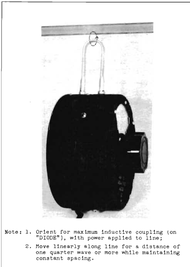
Figure 10 - CHECKING FOR STANDING WAVES ON TRANSMISSION LINES
